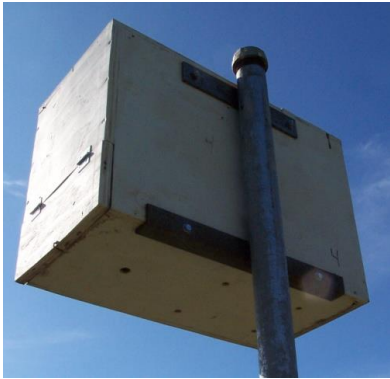
Figure 2 Mount by welding piece of angle iron
