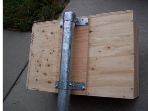
Figure 3. Mount back of nest box with pipe clamps
